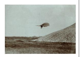
To glide, he ran and jumped off a hill with the air passing over the wings providing lift against the falling force due to gravity.
